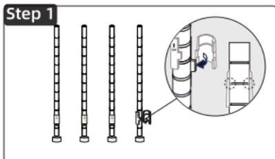
Take out the four bottom pole with feet. Secure the plastic clips at the same height on each pole. It will utter a sound while installing well the clip. (Set the height according to your needs, making sure the "TOP" side of the clip faces up.)
