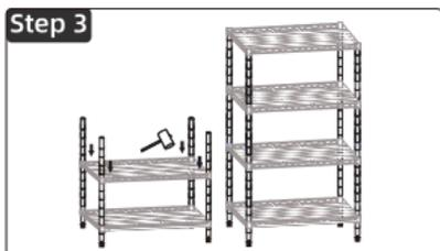
Use the four middle poles to spiral tighten clockwise with the bottom poles. Repeat the previous steps to install the second and subsequent layers.
