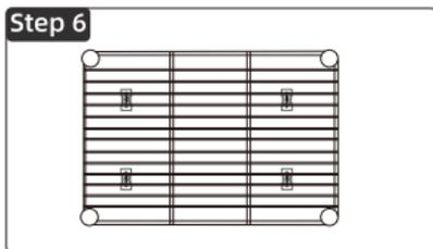
Thread plastic ties through the metal clips and secure the clips to the wire mesh.
