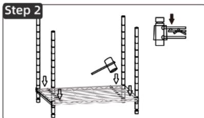
Slide the wire mesh onto the four poles, stand it up, and gently tap the connections to secure them.
