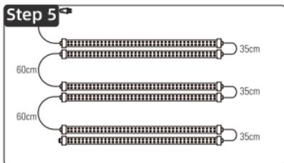
Connect the lights as shown, ensuring the correct positioning of the 35 cm and 60 cm connection cables. Install the waterproof cap on the last light bar.
