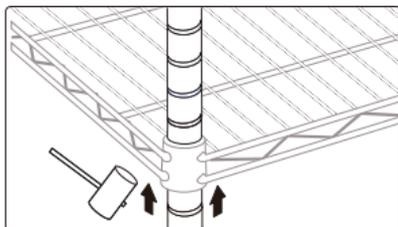
Disassembly Method: Gently tap upward on the four corners of the sleeve to remove the wire mesh panel.
